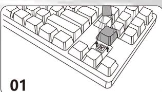
01 Remove the keycaps with the keycap puller.
