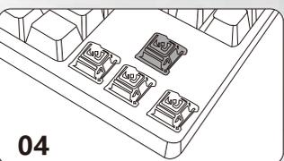
04 Place the switch on the PCB and integrate it closely.
