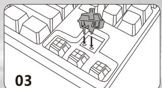
03 Line up the switch pins with the PCB socket.
